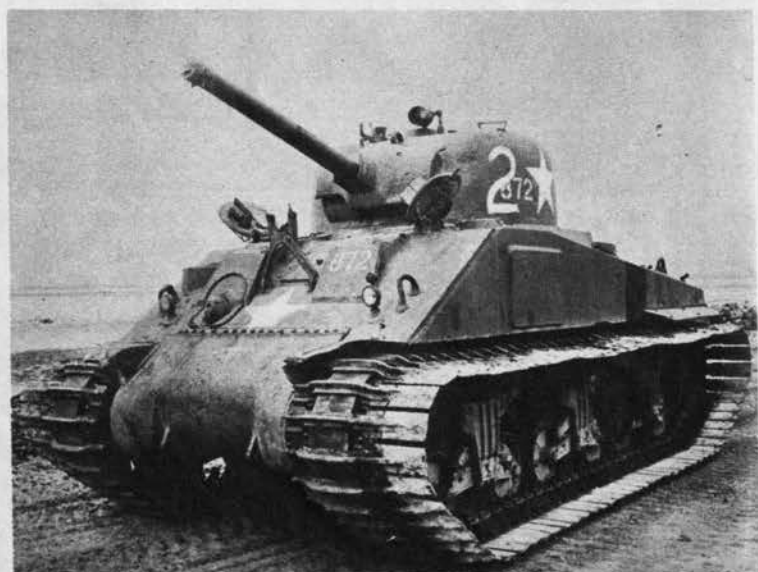
Grousers attached to M-4 track with spaced-out suspension give it over twice standard width, improve performance on marshy terrain.
